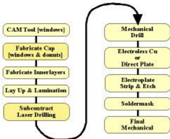
Process Flow Diagram - Foil Cap Lamination
