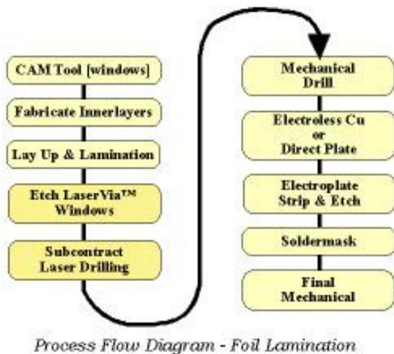
Process Flow Diagram - Foil Lamination
