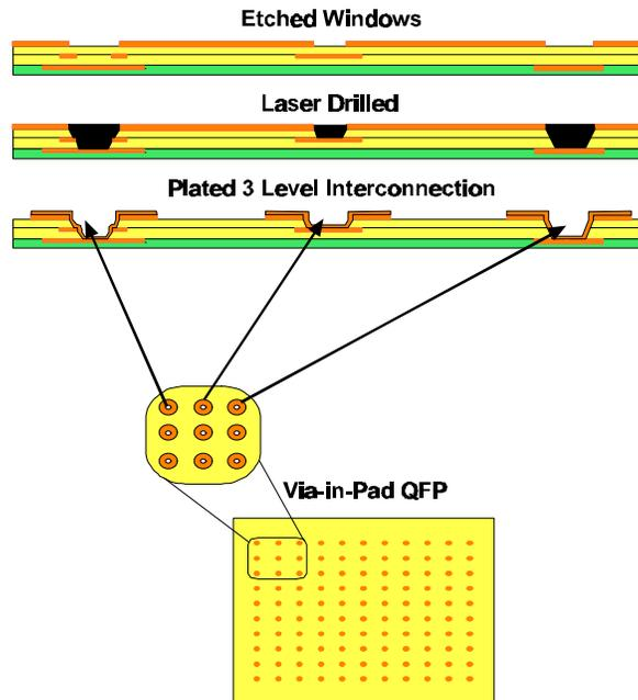
**Fig. 12 BGA Multi-Level Interconnections**
