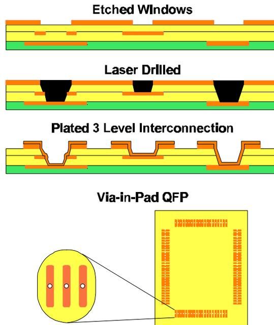
**Fig. 13 QFP Multi-Level Interconnections**
