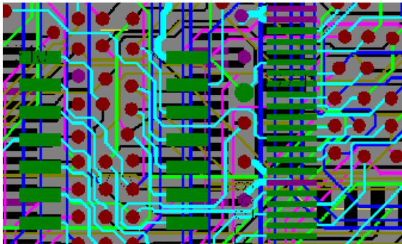
Fig. 6 Via Starvation at the Design Stage
