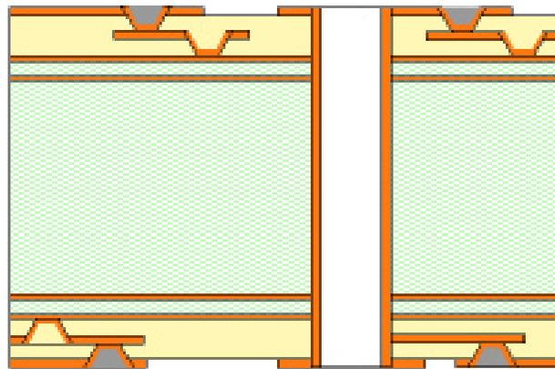
**Fig. 3 Buildup Technology with Staggered Vias**
