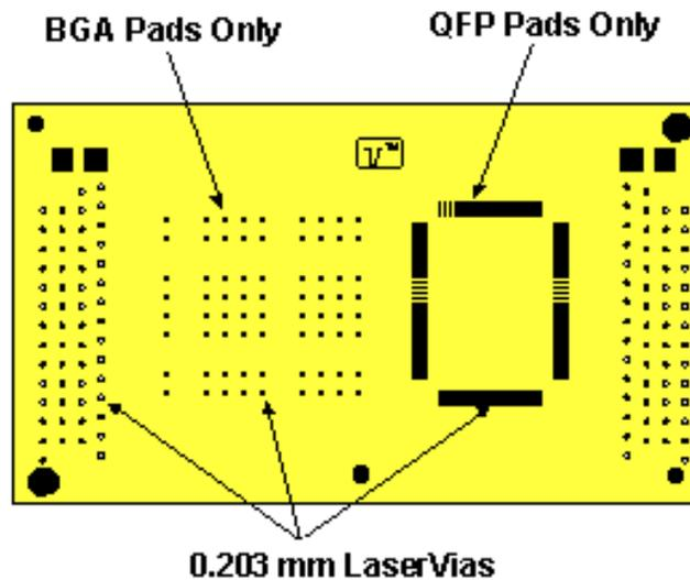
Fig. 8 BGA BizCard Test Coupon
