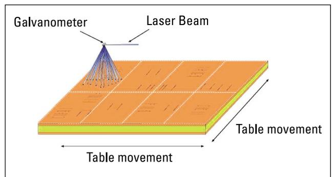
**FIGURE 4b.** Traditional point-to-point laser drilling uses a galvanometer through which the beam is deflected, and the table moves on the X and Y axes.
