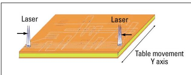
**FIGURE 4a.** The novel method uses a scanning movement in which the laser beam travels on a split X axis and the table moves on the Y axis.
