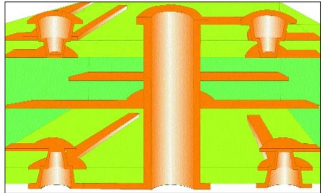
**FIGURE 3.** Although the results are strikingly similar, a significant difference between the variable depth and buildup methods lies in their constructions. Some buildup methods require fabrication and subsequent joining of two PCBs. The novel process (shown here) does not.
