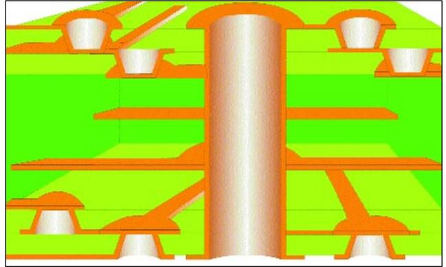
**FIGURE 1.** A typical buildup process yields a staggered blind via interconnect. Compare this to the variable-depth construction in Figure 3.
