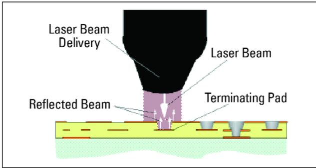
**FIGURE 2.** Positioned over every “window” etched through the top copper surface, the low fluence CO<sub>2</sub> beam ablates the dielectric and is reflected from all copper layers without oxidizing their surfaces.
